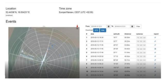
Figure 2. B-finder user panel displays the list of collision events and map of carcass locations.
